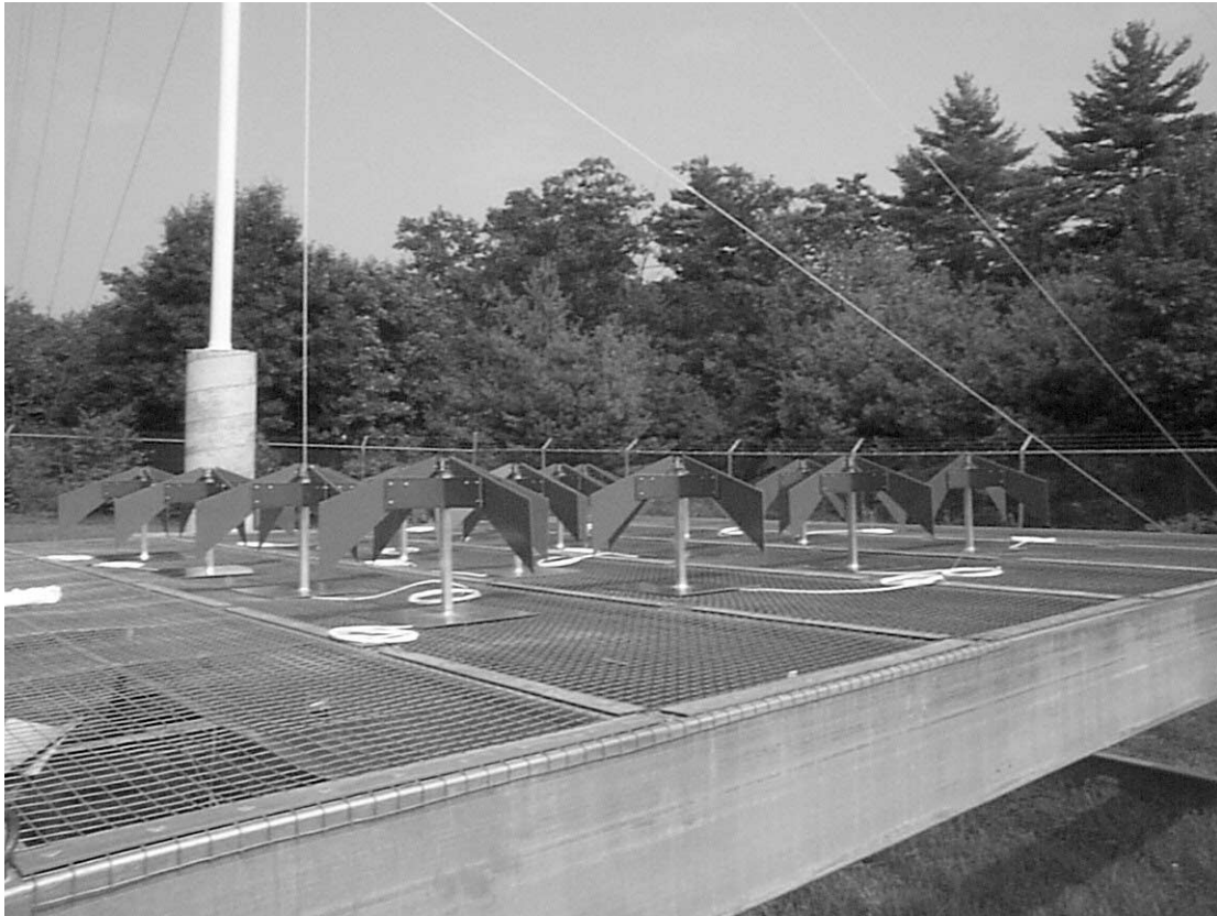
FIG. 1.—Prototype for one 16 element antenna for the 80–240 MHz band.
